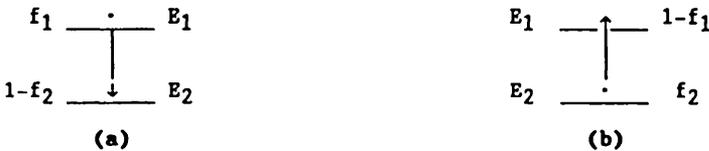
Fig.231.1 The two electronic transition processes between the two energy states or energy levels,  $E_1$  and  $E_2$ , located in a semiconductor volume element  $dx dy dz$  at a position  $(x_1, y_1, z_1)$ .
